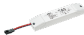
PSU KGP 36W Dali NFC* (50Vf, max. 4 downlights) 108x44x30 mm Expected lifespan 100.000 hrs
